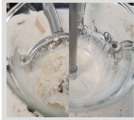
Comparison of the dispersions: on the left inorganic pigment plus C 12-15 Alkyl Benzoate only; on the right inorganic pigment plus C 12-15 Alkyl Benzoate with 5% of Olivem® 2090 (anchor stirrer at 450rpm for 10 mins.)
